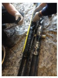
After core inspections and log entries are completed the composite cores are collected into individual, stainless steel bowls, one per dredge prism and NSM, until all composites are collected for each sample. Bowls are covered by heavy-duty aluminum foil between composite inspection and collection procedures.
