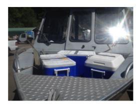
After collection of all composites into bowls is completed for each sample the sediments are completely mixed and placed into the labeled laboratory-supplied sample containers. These containers are then placed into coolers that are supplied with ice to keep the samples at about 4 deg. Celcius. The ice chests were delivered by NRC to the laboratory (ALS), as described and dated in the chain-of-custody.
