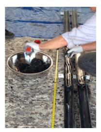
After core inspections and log entries are completed the composite cores are collected into individual, stainless steel bowls, one per dredge prism and NSM, until all composites are collected for each sample. Bowls are covered by heavy-duty aluminum foil between composite inspection and collection procedures.
