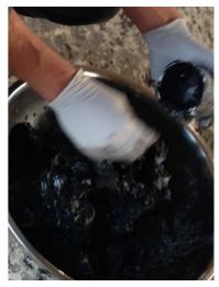
After collection of all composites into bowls is completed for each sample the sediments are completely mixed and placed into the labeled laboratory-supplied sample containers. These containers are then placed into coolers that are supplied with ice to keep the samples at about 4 deg. Celcius. The ice chests were delivered by NRC to the laboratory (ALS), as described and dated in the chain-of-custody.
